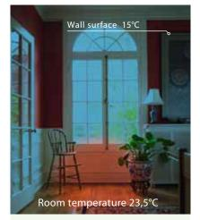
Before internal insulation: Cold walls – uncomfortable even with high internal temperature
