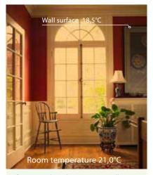
After internal insulation: Warm walls make for a comfortable room climate even at lower temperature
